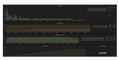
kafka-connect-fluentd CPU usage is less than 20%
